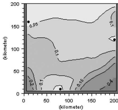
Fig. 8. Spatial distribution of RMSE values between the true run and the 100 EnKF run for the wind error case. The positions of the measurements are indicated by dots.
