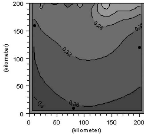
Fig. 2. Spatial distribution of RMSE values between the true run and the false boundary run, where a realisation of the Gaussian process described by Table 1 has been added. The positions of the measurements are indicated by dots.
