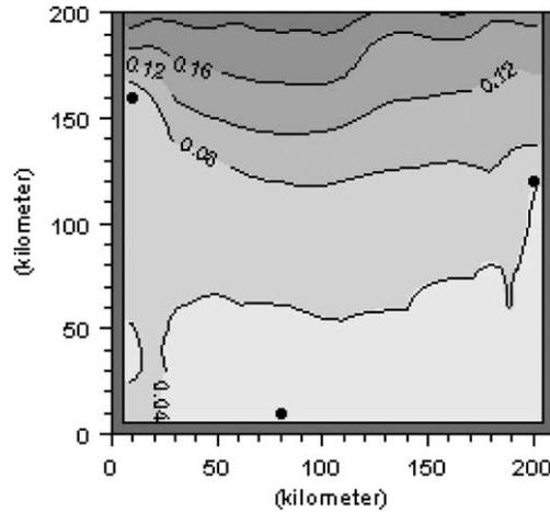
Fig. 7. Spatial distribution of RMSE values between the true run and the 100 EnKF run for the boundary error case. The positions of the measurements are indicated by dots.
