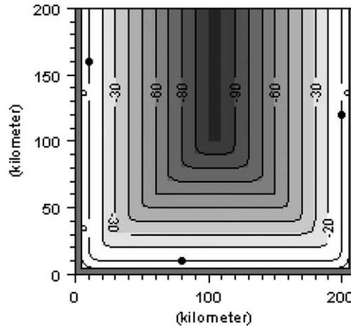
Fig. 1. Bathymetry of Ideal Bay. The three dots indicate the positions, where water level time series were extracted to be used as measurements.
