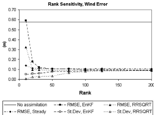
Fig. 5. Sensitivity to rank of error covariance for perturbed wind velocity runs.
