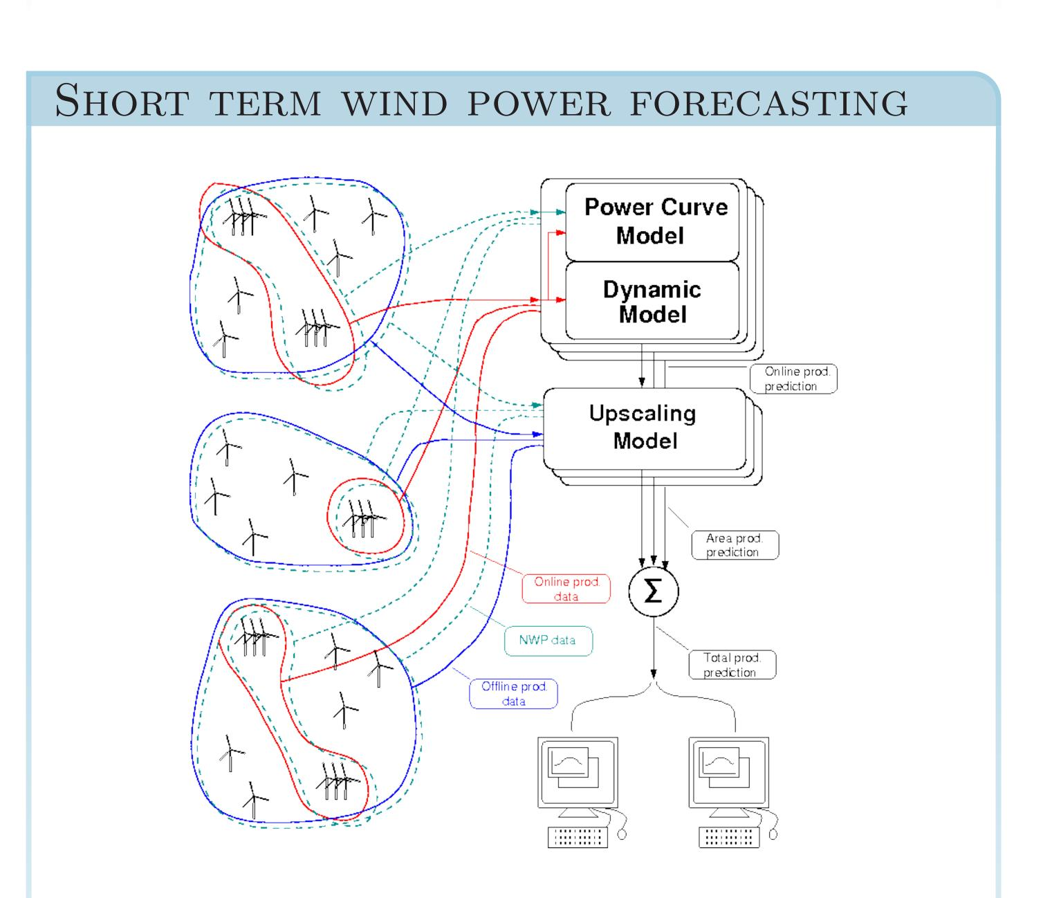
WRF output wind fields will be coupled to a widely used wind power prediction model, namely the Wind Power Prediction Tool (WPPT), maintained by ENFOR A/S; a Danish company that specialises in forecasting and optimisation for the energy sector. This integrated wind power prediction tool will produce scenario forecasts for the coming hours to days, which can then be fed into any type of system model or decision making problem to be solved. Examples of WPPT scenario forecasts are shown below.
