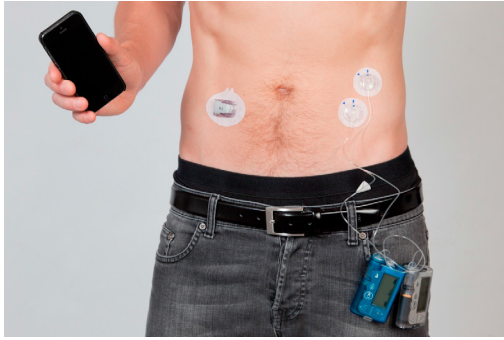
Fig. 1. The dual-hormone artificial pancreas. It includes a CGM sensor, a smartphone for monitoring and control, an insulin pump and a glucagon pump.
