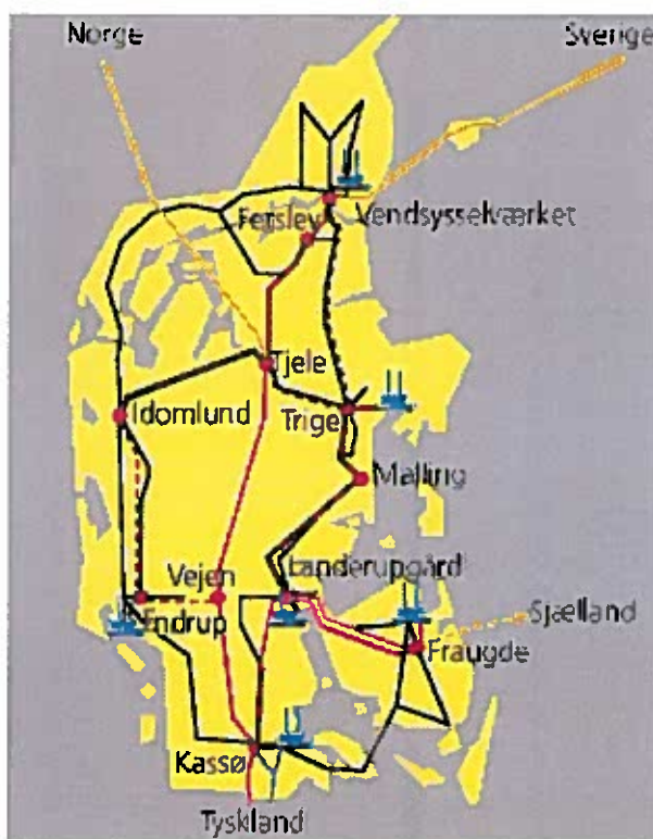
Figure 1: Transmission network and power stations in the Eltra/Elsam supply area.
